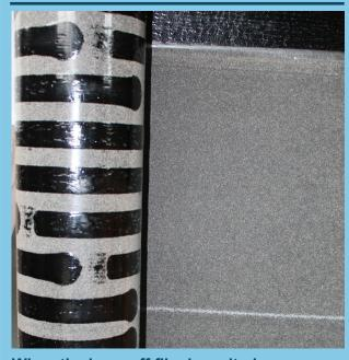
When the burn-off film is melted away, COLVENT's heat activated ribbon strips are adhered to the substrate.
